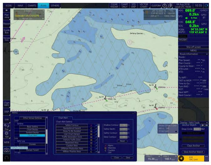
Select Safety Contour in ECDIS and select viewing groups for soundings, seabed features and contours to be displayed. Ensure all obstructions and potential hazards are displayed (safest is to use Display = "ALL")
