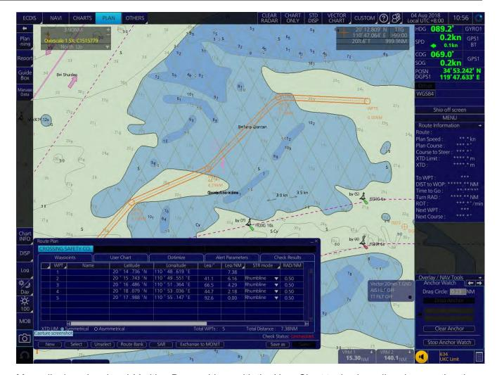
Manually draw (mark-up) Limiting Danger Lines with the User Chart tool using a line demarcating the safe and unsafe areas and marking the latter as Danger. Select the User Chart danger alarm in the Chart Alert window for the manually drawn Limiting Danger Lines (and save) so that any approach to this area alarm is activated.
